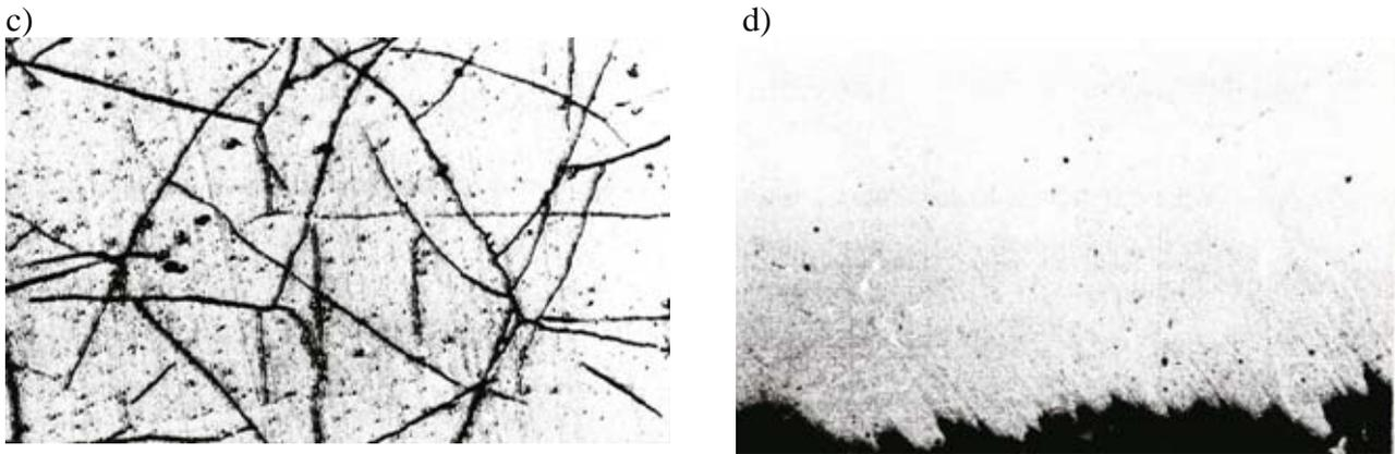
Fig. 9. Structure of electrolytic coating (enlarge. 250x): a) – hard iron, b) – hard chrome – dense crack mesh, c) – hard chrome – sparse crack mesh, d) – hard chrome – no crack mesh
