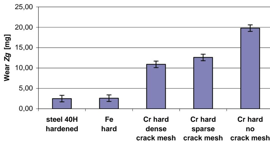
Fig. 4. Mean value of slide bearings wear  $Z_g$  after finish interaction with model and electrolytic coatings
