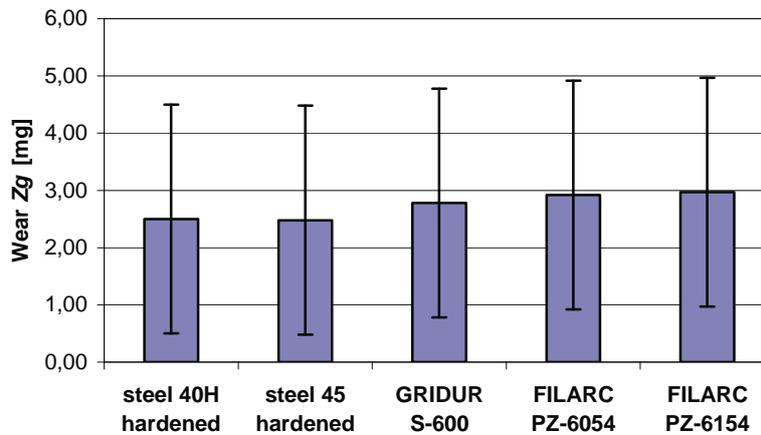
Fig. 1. Mean value of slide bearings wear  $Z_g$  after finish interaction with model and surfaced by weldings
