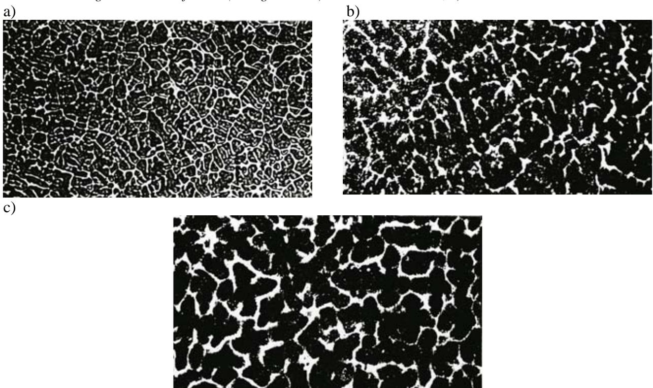
*Fig. 8. Structure of surfaced by welding layer (enlarge 250x): a) – material GRIDUR S-600, b) – material FILARC PZ-6054, c) - material FILARC PZ-6154*
