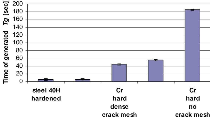
Fig. 5. Time of generated  $T_g$  since the start of generated potential difference effective value  $U_{S-GRP}$  for frictional contact with model and electrolytic coatings
