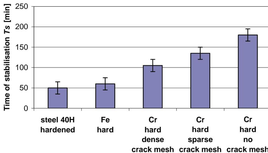
Fig. 6. Time of stabilisation  $T_s$  since the beginning of interaction until stabilization of potential difference effective value  $U_{S-GRP}$  for frictional contact with model and electrolytic coatings
