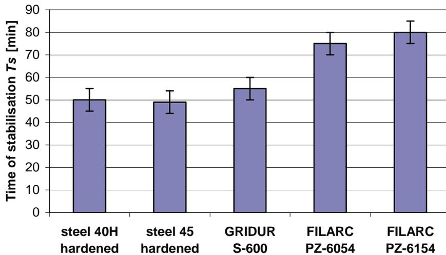
Fig. 3. Time of stabilisation  $T_S$  since the beginning of interaction until stabilization of potential difference effective value  $U_{S-GRP}$  for frictional contact with model and surfaced by weldings
